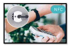
Near Field Communication (NFC) is a short-range wireless technology used between an NFC tag and an Android-powered device, requiring 4cm or less to connect.
