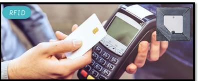
Radio Frequency Identification (RFID) is a wireless system using tags and readers. A reader is a device that sends out radio waves and receives signals back from the RFID tag,
